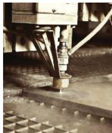
The water cutter is running at almost full capacity – cutting thick plates of titanium with ease.
